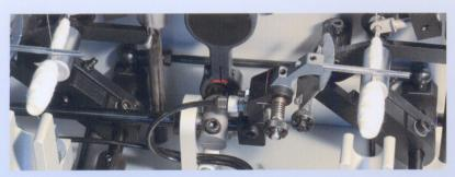
NEW: Individual setting of knotting device on each winding head.
